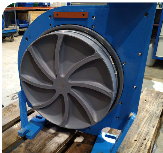
Pump opening after 3 months of operation
